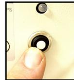
This is a built-in 15 amp circuit breaker. If this breaker trips (sticks out more than normal) the unit must be sent in for service.
