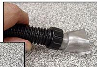
This unique swivel design allows you to active and disable the swivel action. It is all within your control. Do not tighten the swivel collar down all the way and the swivel will rotate during use. If you ever need to disable the swivel, simply tighten the collar down until the swivel action stops. The black swivel connector can be removed from the hose by simply pulling it out of the hose. This may be required if the hose is ever damaged and
