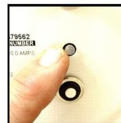
The green light will be on anytime the unit is plugged in and indicates that the system is up and ready to be used. If this light ever turns yellow or red, the unit must be sent in for service.
