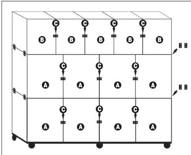
Cage Connectors are designed to work with your existing cage hardware. Unscrew the bolts at the contact points between two cages. Fit the Connector over the two open holes, then screw in the bolts to secure the Connectors in place. Use at least two Connectors for each touching cage side.
