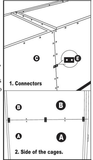
Do not use stacked Cages until they are secured together with Cage Connectors. Shown with optional Large Cage Base (sold separately).
