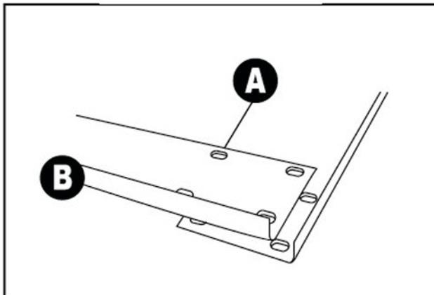
1. Arrange the Front and Back Panels (A) and the Side Panels (B) in a rectangular shape.
