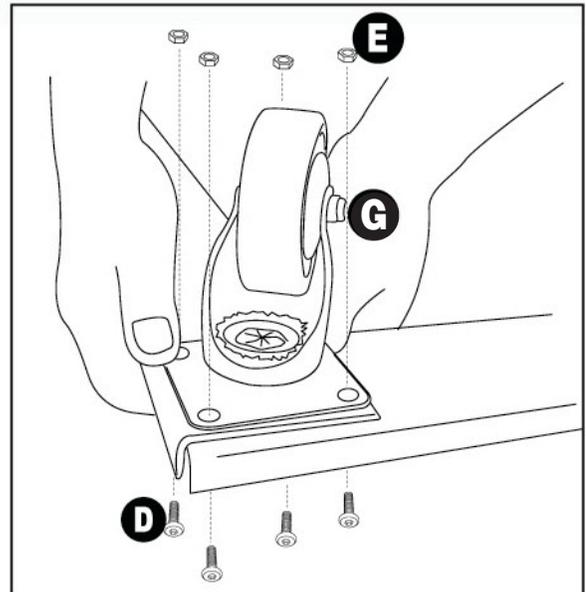
2. Attach the Wheels (G) to each of the four Corners as shown. Use the two Wrenches (C and F) to tighten Bolts (D).
