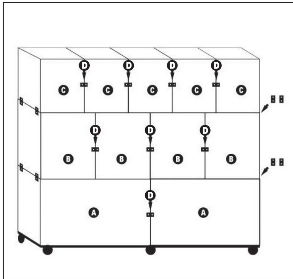
Arrange the five Small cages on the top row, the four Medium Cages on the middle row, and the two Large Cages on the bottom row. Not sold with Cage Base.
