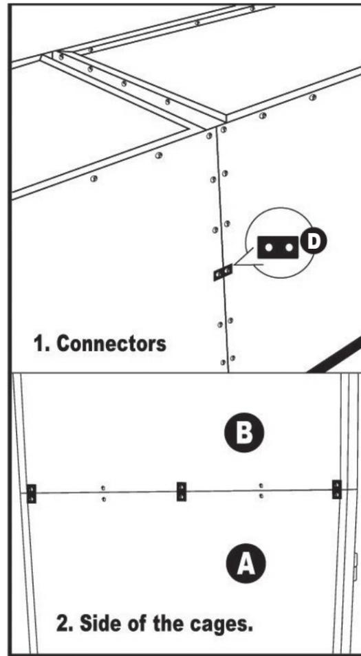
Cage Connectors are designed to work with your existing cage hardware. Unscrew the bolts at the contact points between two cages. Fit the Connector over the two open holes, then screw in the bolts to secure the Connectors in place. Use at least two Connectors for each touching cage side.
