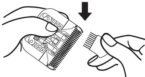
2. Blade oiling: Use 1-2 drops of lubricating oil on the 5 points shown below.
