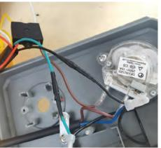
3) Connect the blue power cord with the cut blue cord on the motor, and tape them with black electrically insulating tape. Connect the black power cord with the cut black cord on the motor, and tape them with black electrically insulating tape.
