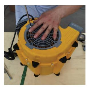
5) Assemble the motor shell.
