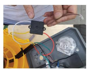
2) Plug the red wire into position 1 of the capacitor. Plug the yellow wire into position 2 of the capacitor. Plug the white wire into position 3 of the capacitor.
