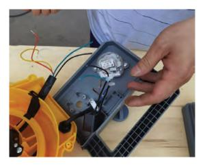
3) Cut the black and green wires on the motor.
