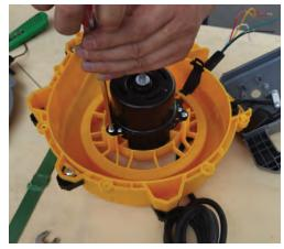
4) Remove the screws holding the motor in place, and the motor can be removed.
