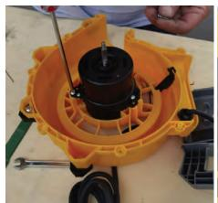
Fix the motor to the bracket with screws and thread the wires through the holes in the shell for fixing.
