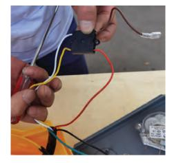
2) Unplug the red, white, and yellow wires from the capacitor of the motor with a screwdriver.
