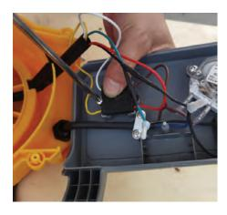
Screw the black capacitor in the original position on the panel.
