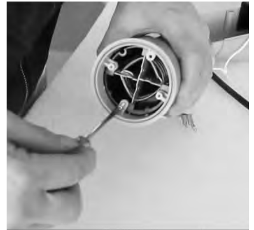
10) Insert new Heating Element in Dryer Tube and secure from front of tube with 2 screws.
