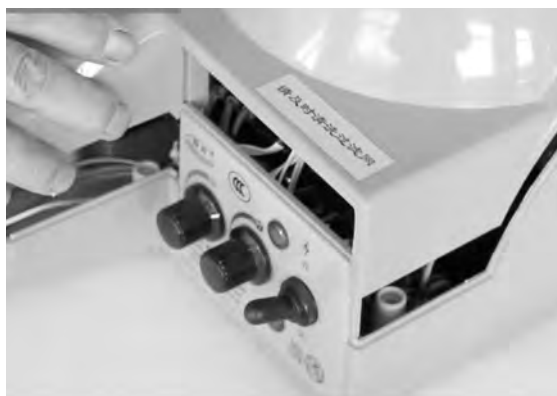
15) Replace Dryer Cover and Dryer Tube secure with screws.
