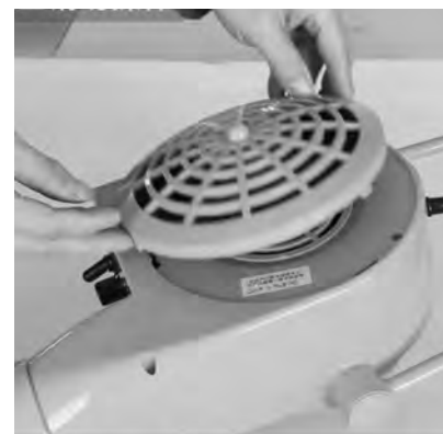
16) Replace Filter and Filter Holder, turn clockwise to lock in place.
