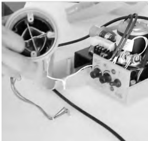
10) Insert new Heating Element in Dryer Tube and secure from front of tube with 2 screws.
