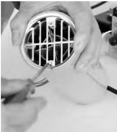
11) Replace front metal retaining guard and secure with 2 screws.
