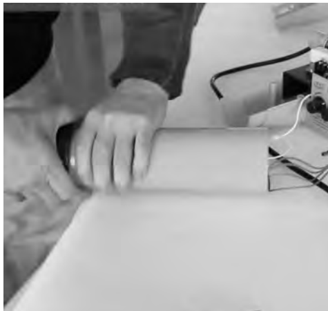
12) Replace nozzle on front of tube and replace retainer clip
