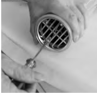
7) Remove Screws from front guard on the Dryer Tube.
