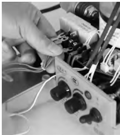
13) Reconnect wires to wire posts and tighten screws.
