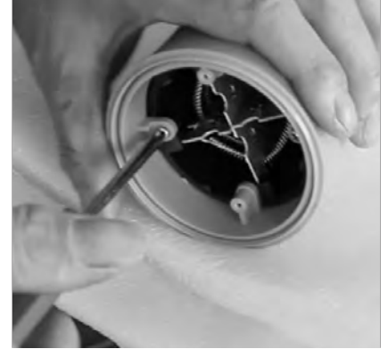
8) Remove retainer screws on tube holding heater element in place.
