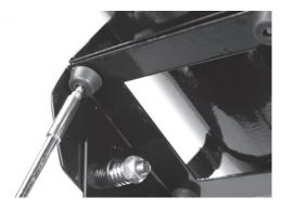
7. Attach the dryer body (G) to the metal frame on the top pole using the four rounded screws with rubber feet (H). Use a Phillips screwdriver to tighten the screws.
