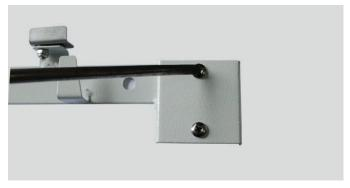
Attach the large metal bracket (E) to the wall (at the appropriate height) using the large screws (C) with the plastic screw anchors (D). You will need to first mark your two holes on the wall and then drill the holes so that the plastic screw anchors (D) can be placed within. Repeat the same action as above with the small metal bracket (F).
