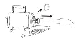
After each use, remove the C-shaped clip and remove the Blower Tube from the dryer.
