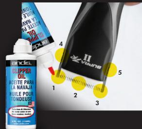
**HOW:** With the tool running, place 3 drops of oil across the teeth of the blade and 1 drop on each back rail. Turn off the clipper or trimmer and blot excess with a clean, dry cloth.
