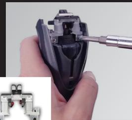
**HOW:** Turn off clipper and snap off the detachable blade. Slide off blade drive cap. Remove screws with a Phillips screwdriver and lift out drive assembly. Insert new blade drive and reverse steps to complete.
