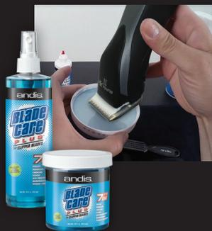
**HOW:** Turn off clipper or trimmer and pour approximately 1/8"-1/4" of Blade Care Plus into the lid or shallow pan. Dip blade only into solution for 10 seconds. Remove and wipe off excess with a clean cloth.
