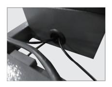
**8.** Return rubber gasket to control box housing.
