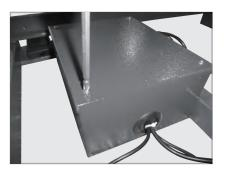
Replace the Control Box Housing Cover and secure in place with screws.
