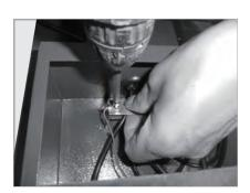
9. Secure wires and cord in Retainer and tighten screw. Secure Ground wire to 2nd screw and screw in place on retainer.
