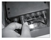
**3.** Unplug the controller and electrical cords from the control box.
