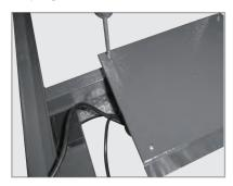
Using a Phillips head screwdriver or drill bit, remove screws holding Control Box Housing Cover in place.
