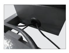
Remove rubber gasket from the Control Box Housing and slide over the electric cord plug. Slide Electric cord plug though hole to inside of housing.
