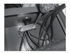
Loosen screw holding wire retainer in place. Remove screw holding Ground Wire and cords in place.
