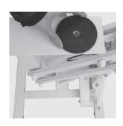
5. Place the Large Plastic Washer **(D)** onto the top of the Pump Base **(B)**.
