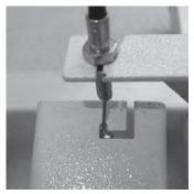
2. Attach the control switch for the gas spring on the pump base (B) to the notch on the pedal from the table base (C).
