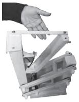
1. Remove this support bar by removing the two Bolts.
