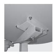
6. Place the Table Top (A) onto the top of the top of the Pump Base (B), sliding the bolt through the Plastic Washer (D) and the top of the Pump Base (B) as shown. Put the Washer, Spring Washer and Nut (E) on bolt of Table Top (A). Tighten with a Standard Wrench.
