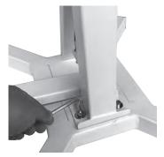
3. Insert two Hexagon Bolts #8x15mm (H) into holes through Pump Base (B) into Table Base (C). From Underneath, add Washers #8 (F) and Nuts #8 (G) to each Bolt and tighten using Standard Wrench and Allen Wrench (J). Tighten underneath with Standard Wrench.
