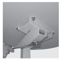
5. Place the Table Top (A) onto the top of the top of the Pump Base (B), sliding the bolt through the Plastic Washer (D) and the top of the Pump Base (B) as shown. Put the Washer, Spring Washer and Nut (E) on bolt of Table Top (A). Tighten with a Standard Wrench.
