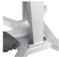
2. Insert two Hexagon Bolts #8x15mm (H) into holes through Pump Base (B) into Table Base (C). From Underneath, add Washers #8 (F) and Nuts #8 (G) to each Bolt and tighten using Standard Wrench and Allen Wrench (J). Tighten underneath with Standard Wrench.
