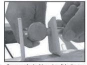
Remove the locking pin, slide the top of the electric lift shaft into place between the mounting brackets, and reinsert the locking pin through the mounting brackets and the top of the electric lift shaft.
