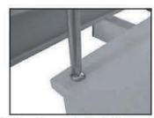
15. Place the cover back onto the electrical control box. Using a Phillips-Head screwdriver, replace the screws and tighten to secure in place.
