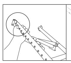
Depress locking pin on outside of leg to release
