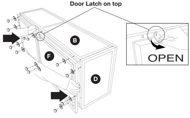
Attach Door Handles (A) using provided Screws (I) and Washers (J); tighten from inside with a Phillips Head Screwdriver.
