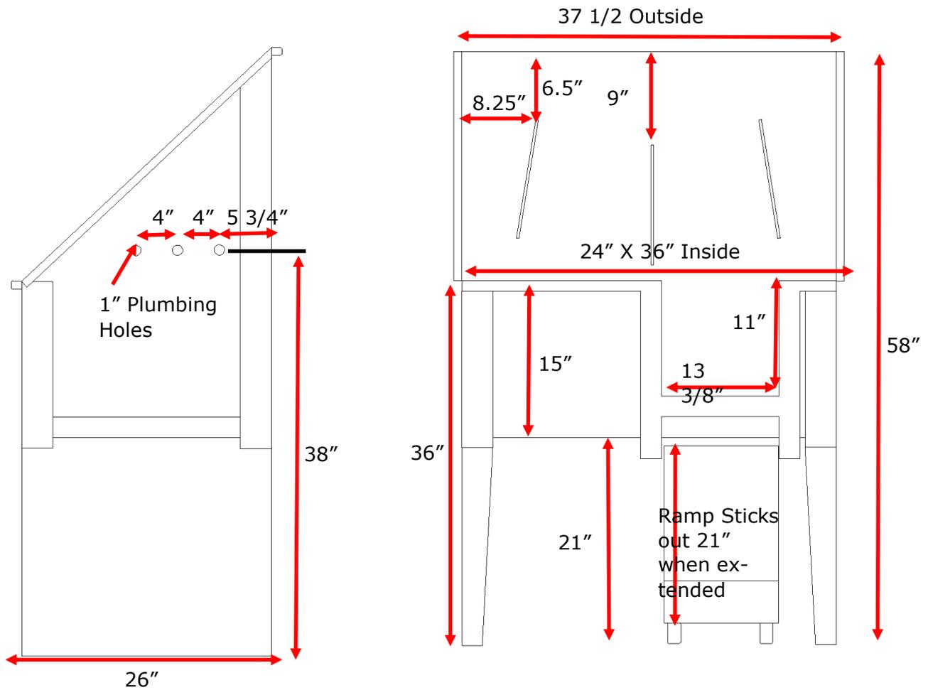
Available as Left, Right or center drain. 3.5" drain hole, located 7" on center from the left or right.
