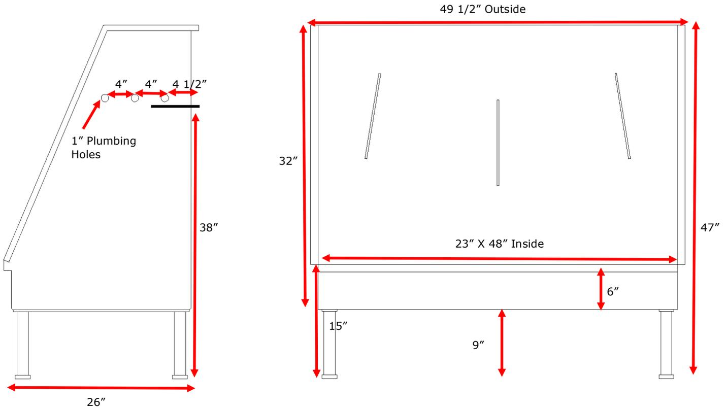
Available as Left, Right or center drain. 3.5" drain hole, located 7" on center from the left or right.
