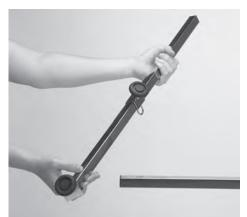
9). Find the Subsidiary Grooming Arm (C) and slide it 10). Re-attach the fastener you took off onto the Major Grooming Arm (B). Slide it to the middle of the Major Grooming Arm (B) and then secure it by tightening the fastener.
