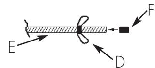
5. At an angle, press the Threaded Rods with attached Foot Support Inserts into two of the Support Feet (G).
