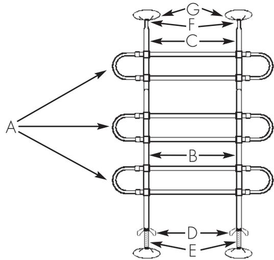
1. Insert Vertical Upright Tubes (B) through the upright support brackets on two of the Telescoping Horizontal Tubes (A).
