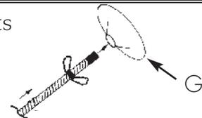
6. Take the Threaded Rod/Support Foot assemblies from Steps 4 & 5 and connect them to the Vertical Upright Tubes (B).
