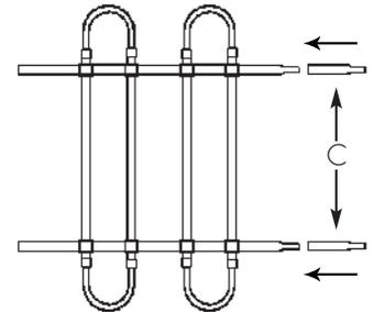
3. Attach the remaining Telescoping Horizontal Tube (A) to the ends of the Vertical Upright Tubes (B).
