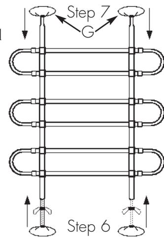
8. Place the Barrier in your vehicle with Threaded Rod Assembly portion against the floor, and extend the barrier vertically until it fits snugly against the floor and roof of the vehicle. Use the Wing Nuts (D) to make adjustments.
