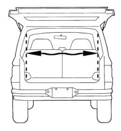
Remove the Threaded Rods (D) from the tubes on the Main Barrier Sections (A) and set them aside. Identify the left and right main panels by placing the panels on the ground with the tubes down. Attach the Short Rubber Tube Sound Dampeners (K) to the Left Barrier Panel to eliminate any possible vibration rattles.
