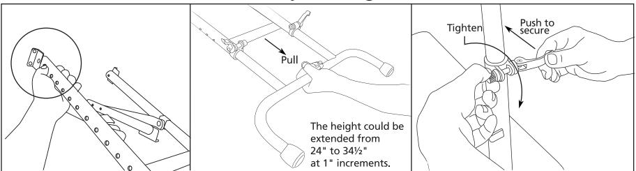
Depress locking pin on outside of leg to release
